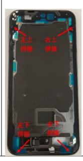
If excess adhesive is applied and overflows internally, remove it using a prying tool. For uneven glue application, adjust the dispensing path with the needle to ensure uniform coverage. Finally, peel off all release films from the double-sided tapes.
