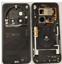
Do not to touch the rear cameras or the lens of the back cover with your fingers or any foreign objects, and avoid damaging nearby components.
