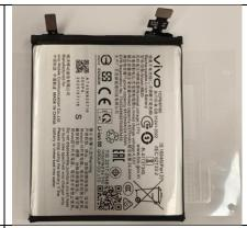
Step 4: Before installation, ensure the battery and battery compartment are free from any foreign objects. Pace the battery into the main upper part, and press firmly on adhesive areas indicated by the blue frames to activate the adhesive.
