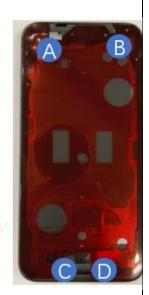
Step 3: Apply glue to the four corner joints. Before application, clear any cured glue from the needle tip to ensure proper glue flow. (After spreading, make sure the glue fully bonds the two parts and does not leak onto the frame.)
