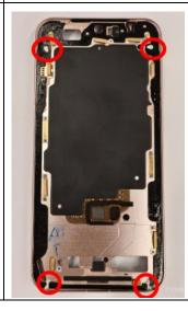
Step 4: Insert the display FPC into the frame's FPC slot as shown. Prealign the display screen and gradually press it into place, ensuring proper alignment.
