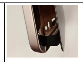
Step 5: After installing the display, wrap your fingers in a lint-free cloth and press firmly around all adhesive and glued areas for 1 minute to activate the adhesive and secure the bond.
