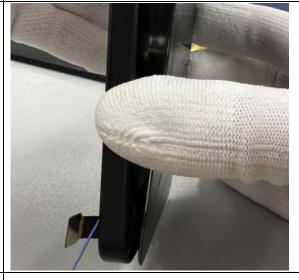
Step 6: Wipe excess glue from the bottom edge with a lint-free cloth.
