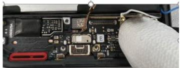
Step 2: Secure the BTB connector of the FMA board to the ANA board.
