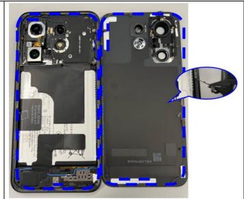
Avoid touching or leaving debris on rear camera lenses or the lens protector. Take care not to damage nearby components.
