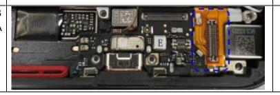
Step 3: Connect the coaxial cable and all BTB connectors.
