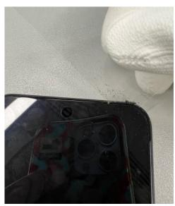
Step 9: After separating all edges, gently remove display by lifting it upward. Note: You need to remove the flexible printed circuit (FPC) in the lower left corner through a slot.
