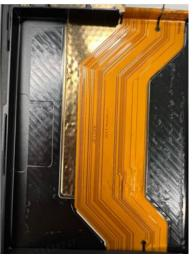
Step 3: Take a new battery PET film. Peel off Liner 1 and attach the exposed PET film to the battery.
