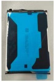
Step 4: Take a battery compartment adhesive tape and apply it to the position as indicated.
