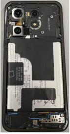
Step 2: Align the back cover precisely and press firmly onto the middle frame. Wrap your fingers with a lint-free cloth and press adhesive areas to activate bonding.
