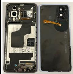
Step 9: Clean residual adhesive from the device frame and back cover using pointed anti-static tweezers or fingers.
