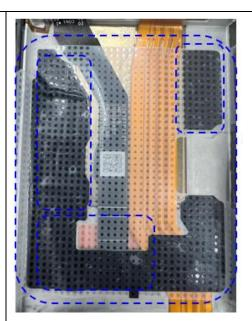
Step 3: Take a new battery PET film and two battery adhesive tapes. Apply them to the battery and main upper part as indicated. Remove all release liners.
