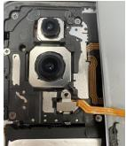
Step 7: Remove the flash connector using anti-static tweezers (lift from the connector's bottom edge).
