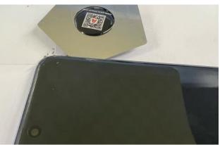
Step 7: After separating all edges, gently remove the display by lifting it upward.
