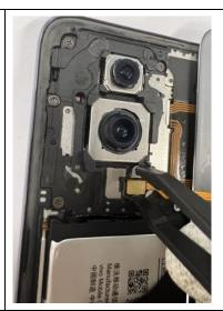
Step 8: Fully separate the back cover from the device.
