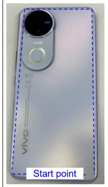
Do not insert the pry pick deeper than 5 mm to avoid damaging internal circuits.
