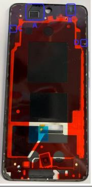
Step 3: Take a bottle of glue, clear any cured from glue the applicator tip to ensure proper glue flow, and apply glue on the bottom edge of the device.
