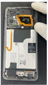
Step 5: Insert and tighten all 17 screws to complete the reinstallation of the frame.
