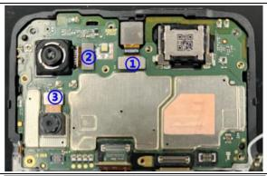
Step 3: Connect the display BTB connector and coaxial cables in the indicated order, and then connect the battery BTB connector.
