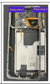
Step 4: Install the frame. Press the frame clockwise to ensure full engagement.
