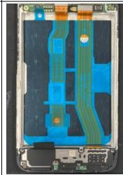
Step 4: Take a new battery PET film and apply it to the battery as indicated.
