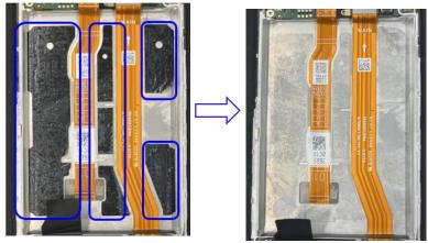
Step 3: Apply the battery back adhesive.
