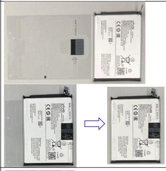
Step 5: Remove the release liner of the battery adhesive tape and install the battery into the compartment. Press the indicated adhesive areas with your fingers to activate bonding.
