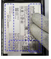
Before installation, make sure that the battery and battery compartment are free of foreign objects.
