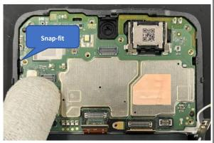
Step 2: Install the camera. Make sure that the camera BTB connector is reliably connected.
