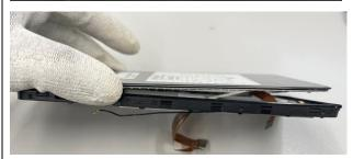
Step 8: Remove the display module.
