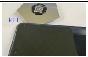
Step 7: After separating all edges, gently remove the display by lifting it upward.
