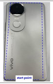
Do not insert the pry pick deeper than 5 mm to avoid damaging internal circuits.
