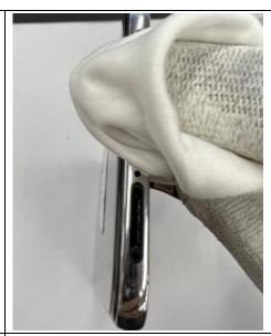
Step 7: After assembly, wrap your fingers with a lint-free cloth and firmly press along all adhesive areas for 1 minute to activate bonding.
