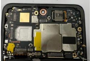
Step 2: Reinstall the camera, and all BTB connectors and coaxial cables.
