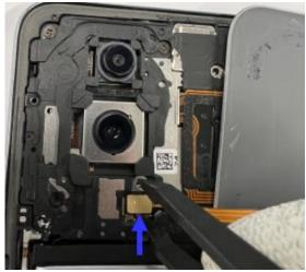
Step 8: Fully separate the back cover from the device.
