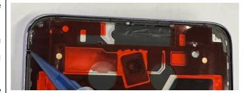
4: Clean Step excess glue inside with a pry tool. Adjust uneven glue with the applicator tip. The figure on the right side shows how it looks after proper glue application. Then, remove all adhesive release liners.
