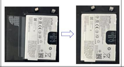
Step 4: Adhere the battery backing tape to the battery as shown in the picture and then peel off the blue release film.
