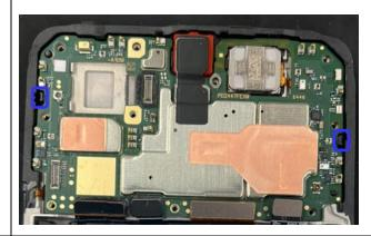
Step 2: Install the camera, and all BTB connectors and coaxial cables in the indicated order.
