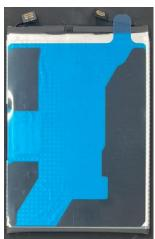
Step 5: Before installation, make sure that the battery and battery compartment are free of foreign objects. Install the battery into the compartment and press the indicated adhesive areas with your fingers to activate bonding.
