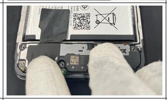
Step 3: Install the middle frame and fasten it with screws.
