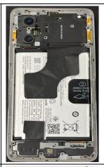
Step 2: Insert and tighten all 16 screws to complete the reinstallation of the frame.
