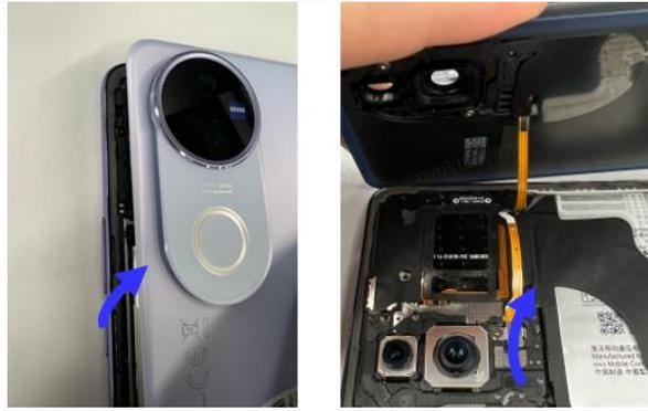
Step 6: Use a screwdriver to remove the screw securing the flash connector's metal bracket, and then remove the metal bracket.
