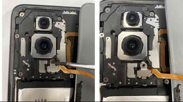
Step 7: Remove the flash connector using anti-static tweezers (lift from the connector's top-right corner).
