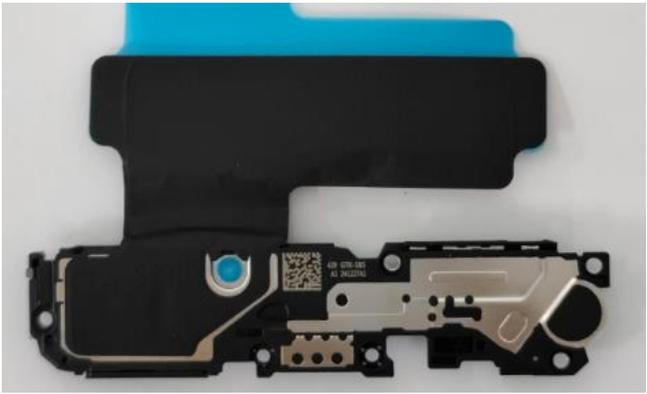
A black plastic speaker component with a blue adhesive strip at the top and a metal mesh grille on the right side. |
