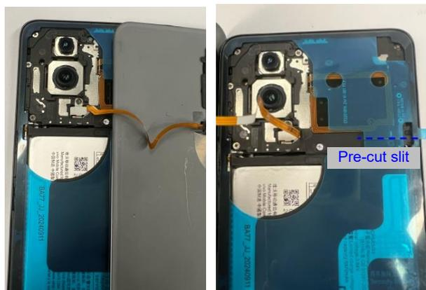
Step 3: Align the back cover precisely and press firmly onto the middle frame. Wrap your fingers with a lint-free cloth and press adhesive areas to activate bonding.
