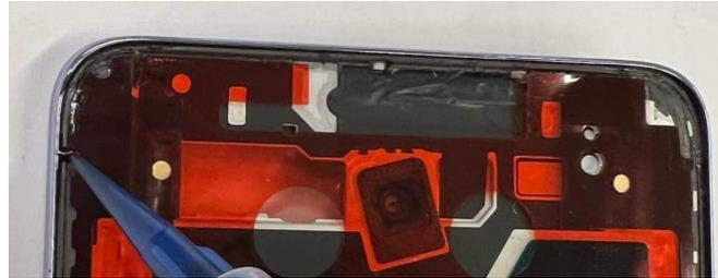
Step 4: Clean excess glue inside with a pry tool. Adjust uneven glue with the applicator tip. The figure on the right side shows how it looks after proper glue application. Then, remove all adhesive release liners.
