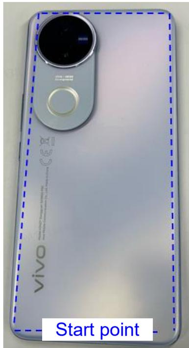
Do not insert the pry pick deeper than 5 mm to avoid damaging internal circuits.
