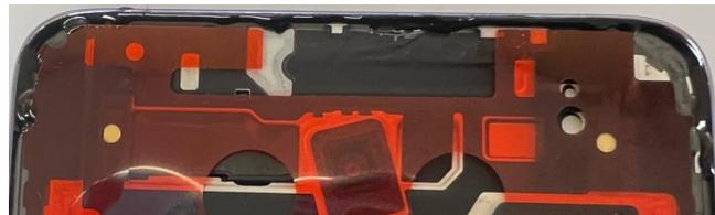
Step 5: Insert the display FPC into the FPC slot in the middle frame, as shown in the figure. Put the display in position, align it with the main upper part, and fully engage them.
