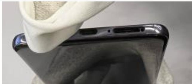
Step 7: After assembly, wrap your fingers with a lint-free cloth and firmly press along all adhesive areas for 1 minute to activate bonding.
