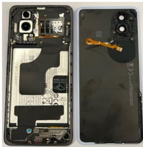
Step 9: Clean residual adhesive from the device frame and back cover using pointed anti-static tweezers or fingers.
