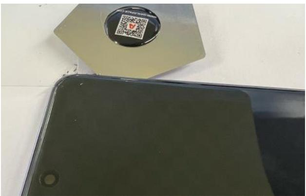
Complete disassembly immediately after heating. Delays may cause cooling and difficulty. Use a metal pry pick only for stubborn areas.
