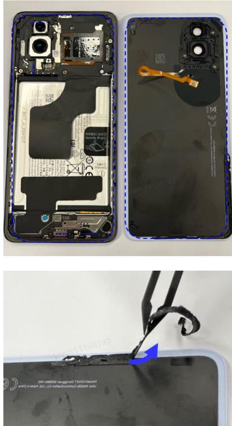
Avoid touching or leaving debris on rear camera lenses or the lens protector. Take care not to damage nearby components.
