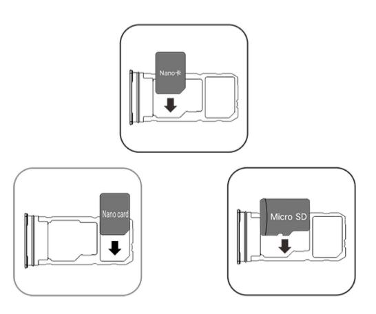
3. With the touch screen facing up, insert the card tray according to the direction of the arrow (with a nano card or micro SD card inserted).
